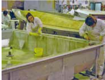
FRP (non-corroding material) manufacture process.
